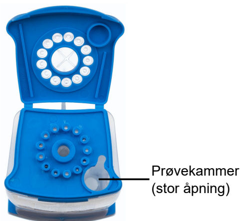
Figur 3. Xpert HIV-1 Qual XC-kassett (sett ovenfra)
