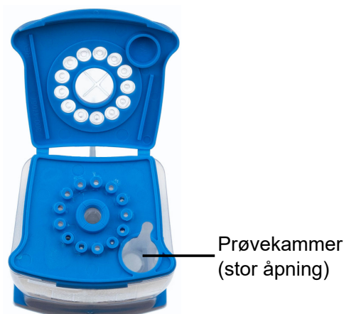
Figur 3. Xpert Xpress GBS-reagenskassett (sett ovenfra)
