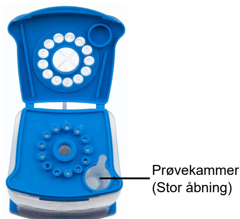
Figur 3. Xpert Xpress GBS-kassette (set ovenfra)
