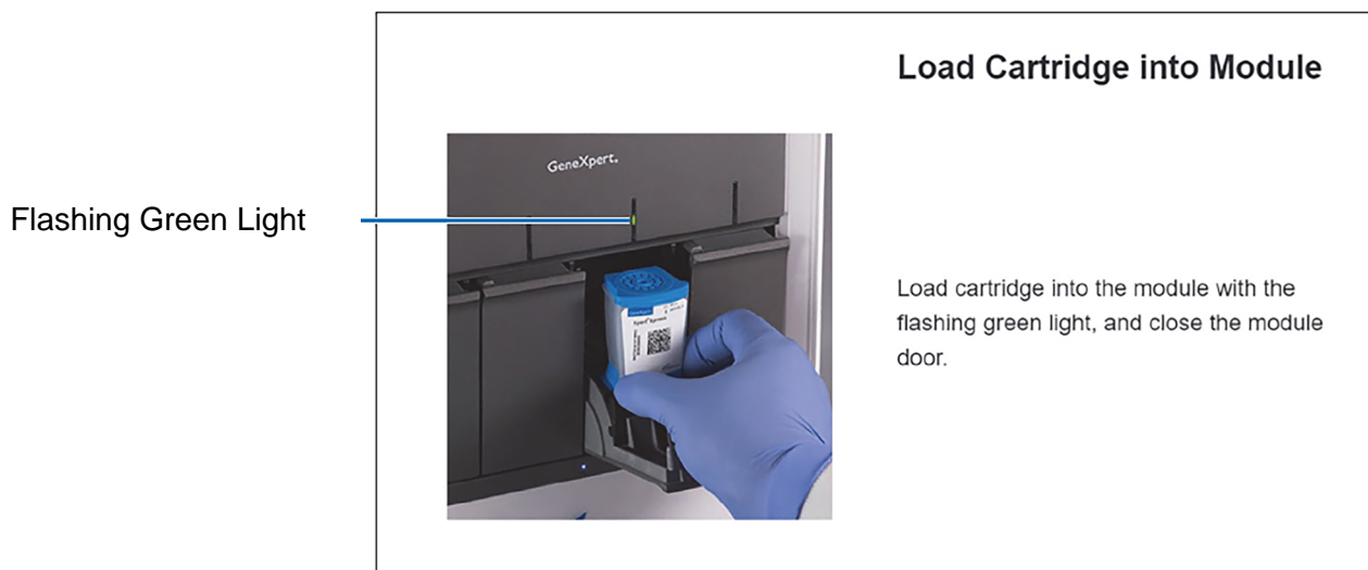
Figure 29. Load Cartridge into Module Screen
