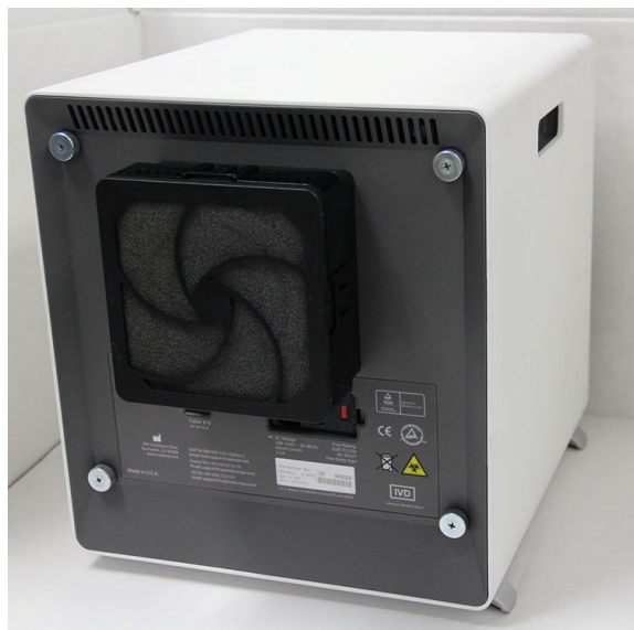
Figure 9-24. GX-IV Instrument Positioned for Access to Filter
