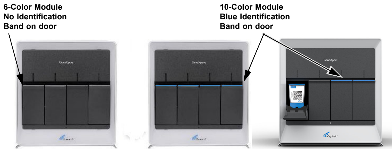
Figure 1-1. Examples of GX-IV Instruments, showing 6- and 10-Color Modules and a Combination of 6 and 10 Color Modules in the Same Instrument
