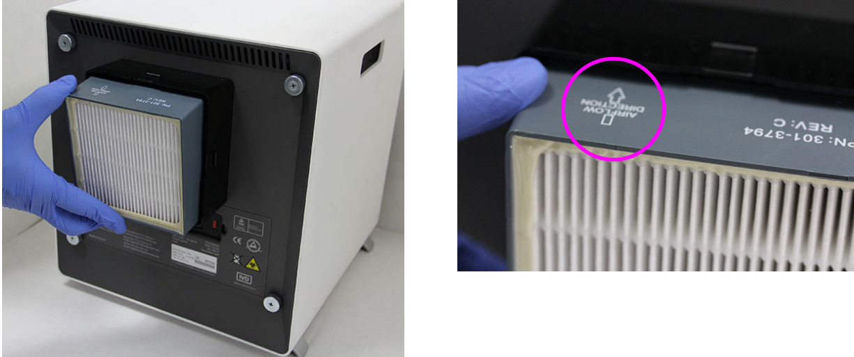
Figure 9-29. Replacing the HE Filter
