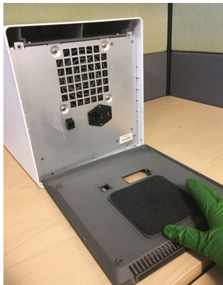
Figure 9-16. Replacing Foam Filter in Older GX-IV
