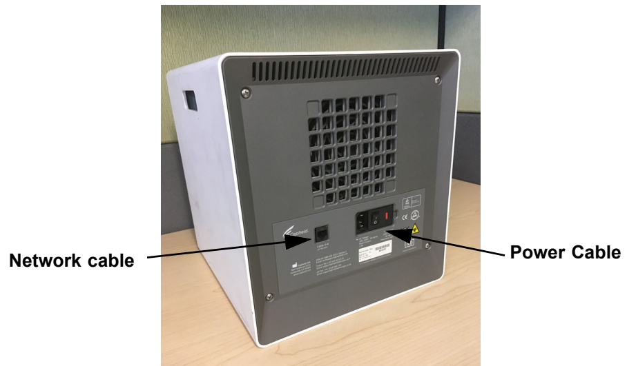
Figure 9-13. Network Cable and Power Cable Locations on Older GX-IV
