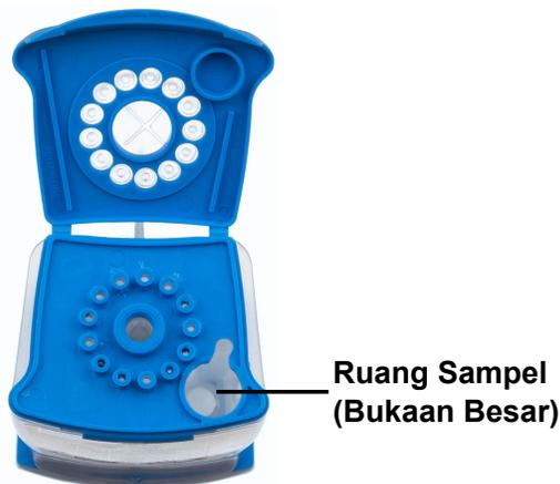
**Gambar 5. Xpert Xpress CoV-2 plus Kartrid (Tampak Atas)**
