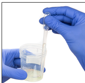
Figure 5. Aspirating to the line on the pipette
