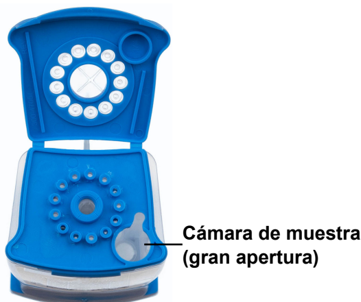
Figura 1. Cartucho del Xpert Breast Cancer STRAT4 (vista superior)
