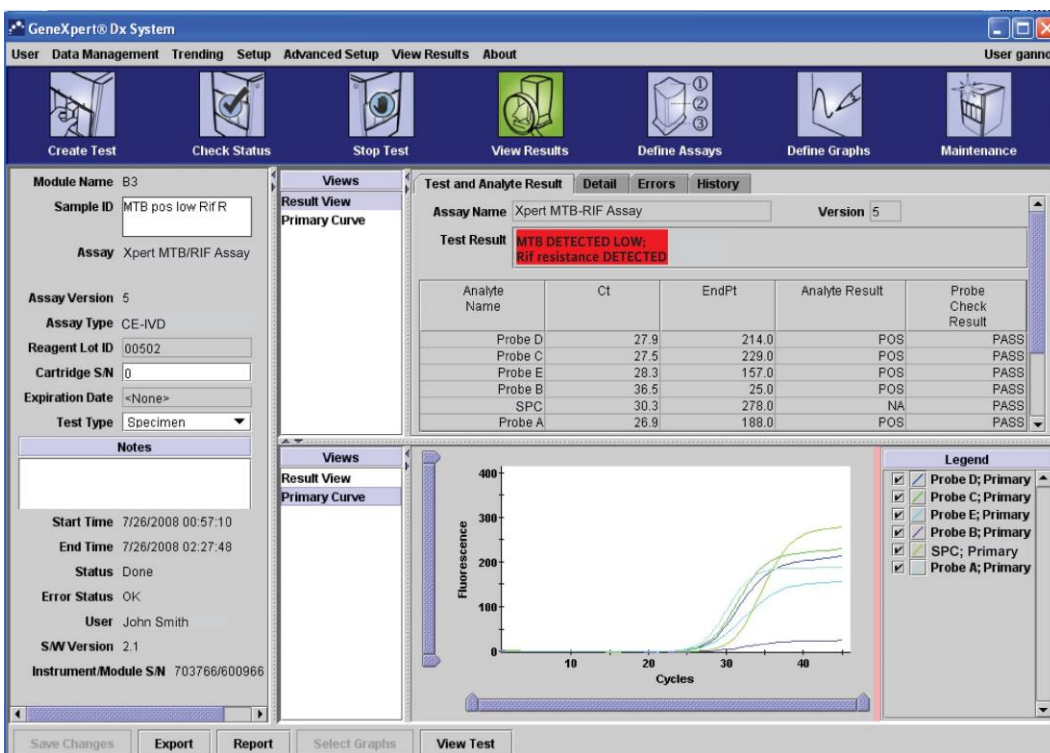
图 2: GeneXpert Dx 系统授权用户结果预览窗口：检测到 MTB，检测到利福平耐药 (MTB DETECTED, Rif Resistance DETECTED)
