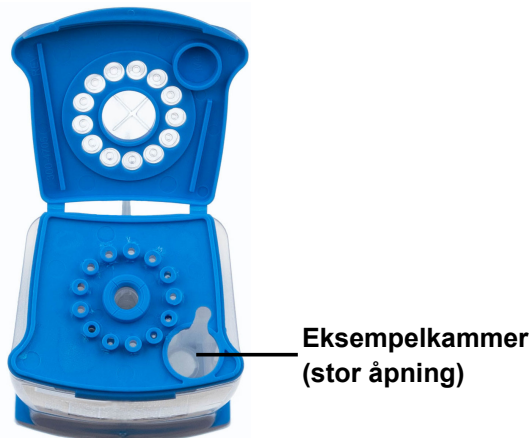
Figur 3. Xpert Xpress GBS-reagenskassett (sett ovenfra)
