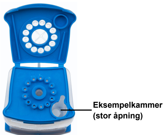
Figur 5. Xpert Xpress SARS-CoV-2/Flu/RSV-reagenskassetten (sett ovenfra)
