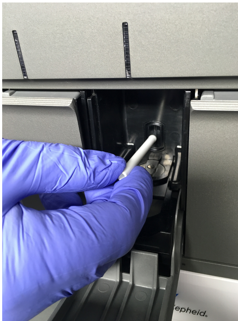
Figure 85. Inserting the Cleaning Brush into the I-CORE Module Slit
