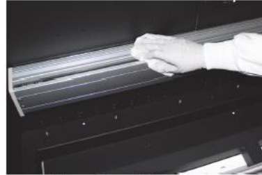
Clean Gantry Rail Covers
