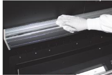
Clean Gantry Rail Covers
